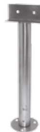
PARTITION BRACE - Stainless Steel Floor Mounted Unit supports 1/2" to 1-1/2" thick panels. Height is adjustable from 11-1/4" to 18" Part No. 9A6005
